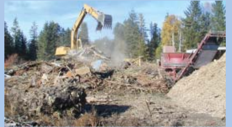
Wood chips from yard and construction waste are used for roadbuilding at the Armstrong/Spallumcheen RDF, windrow composting at the Greater Vernon RDF, and as final cover material at the Lumby RDF.
