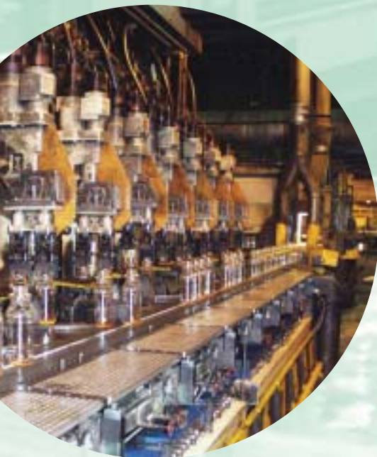
is then fed into a 300-ton furnace, which heats “Gobs” or lumps of molten glass slide down from the furnace and are dropped into specific molds. The resulting bottles or jars take about 45 minutes to cool.
